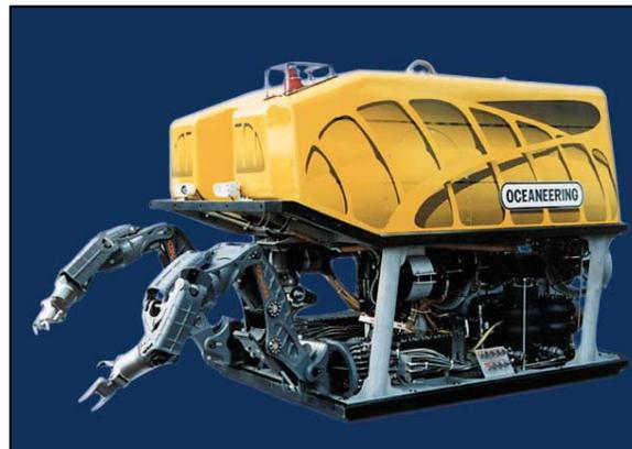
Figure 6-2 Work Class ROV
