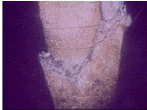
Figure 3-7 Failed Precast Prestressed Pile Due to Delayed Ettringite Formation
