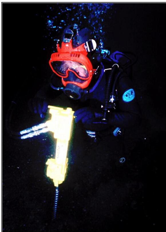
Figure 6-10 Hydraulic Powered Hammer Drill
