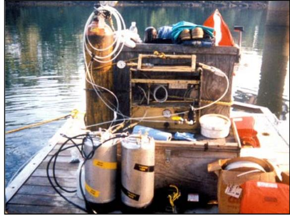
Figure 7-5 Epoxy Injection Equipment on Float
